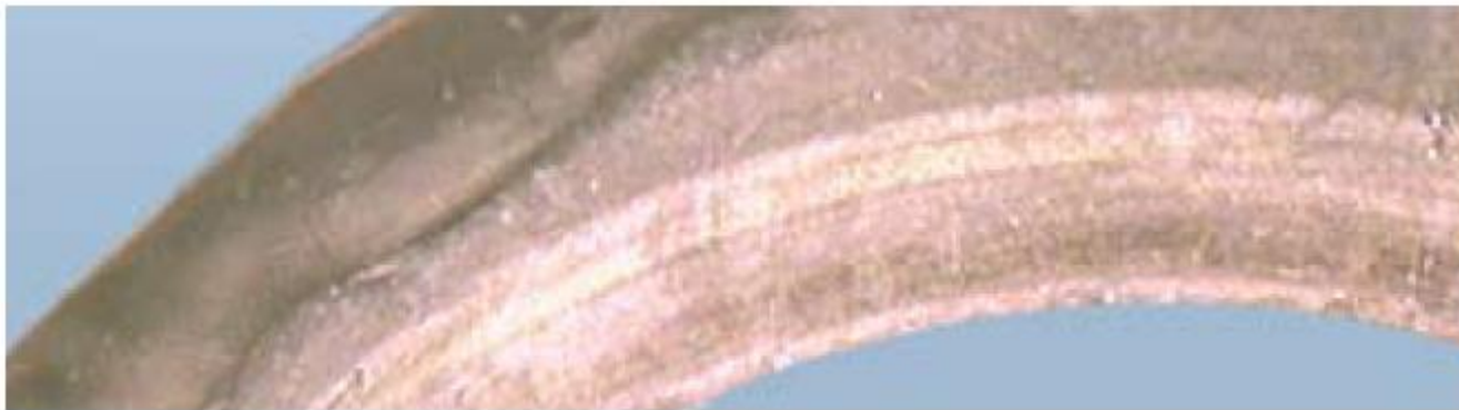
Fig. Selective corrosion in cemented tungsten carbide.
