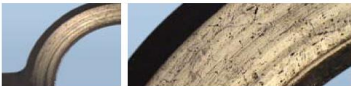
Fig. Normal wear on surface of tungsten carbide seal ring.
