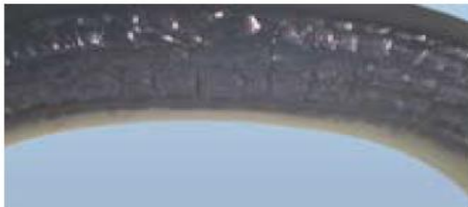
Fig. Surface damage due to high temp. on secondary seals.
