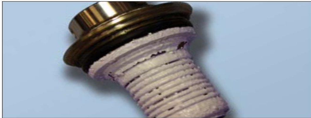
Fig. Metal bellows seal clogged by lime scale build-up
