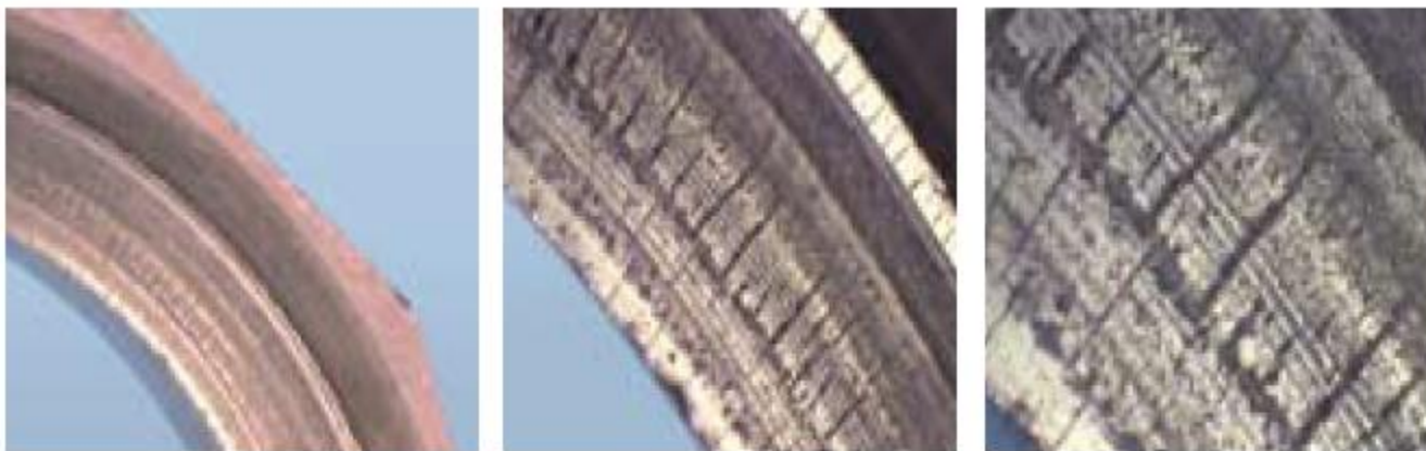
Fig. Severe thermal cracks in seal face caused by poor lubrication
