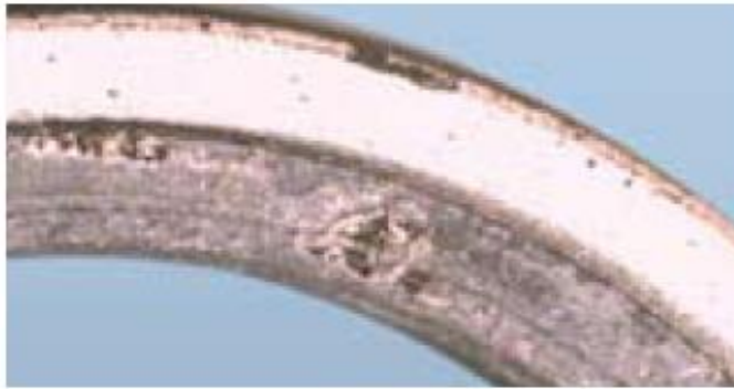
Fig. Deposits on carbon graphite seal face
