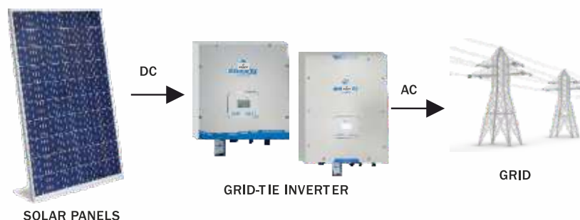
Fig 2.1 Grid-Tie Inverter operation illustration
