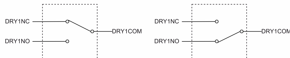
Fig.6 Relay 1 normal and fault operation
