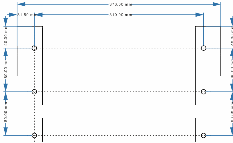
Fig. 5.6 Mounting Brackets for KUSPC - H
