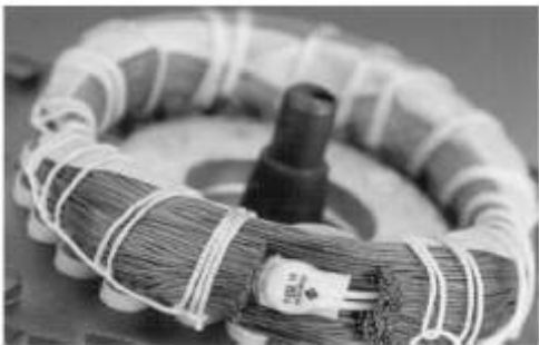
Fig. 21 Motor with Thermal Switches (PTO)
